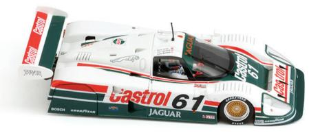
This model featured a carbon fiber monocoque chassis. The engine was a V12 engine with two valves per cylinder. In 1990, displacement was 6 liters for the IMSA version and 7 liters in the Group C configuration; these values were increased in 1991, becoming 6.5 liters for the American version and 7.4 for the European one, whose weight was respectively 930 and 1000 kg.
